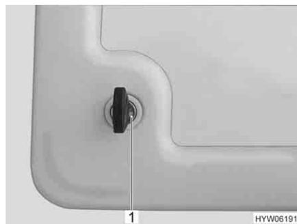
Fig. 36 Push-button lock service flap
