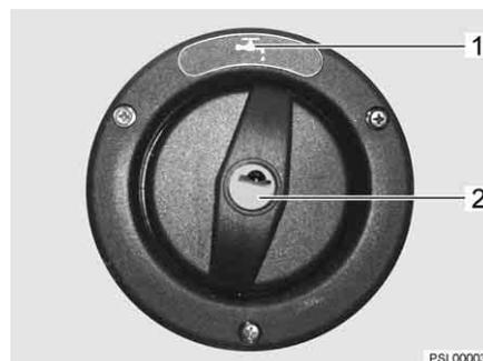
Fig. 220 Cap for the drinking water filler neck (alternative)
