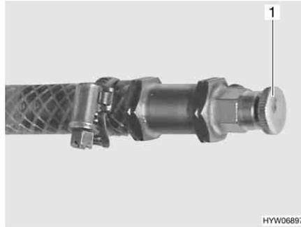
Fig. 268 Bleeding valve of hot-water heater
