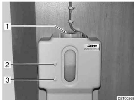
Fig. 267 Compensator reservoir hot-water heater
