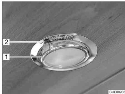
Fig. 275 Recessed halogen light (flat)
