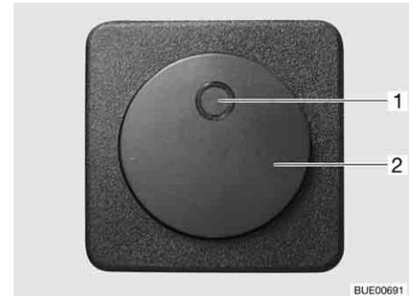
Fig. 187 Switch for electrical floor warming unit
