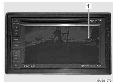
Fig. 17 LCD monitor for reversing camera (example)
