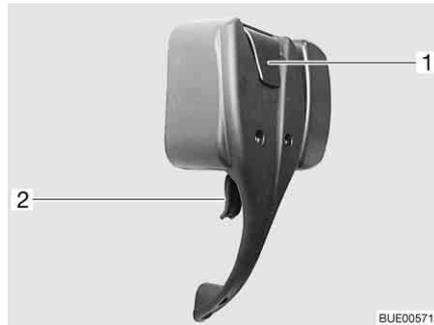
Fig. 30 Door lock of conversion door, inside, locked
