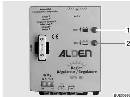
Fig. 156 Solar charge regulator
