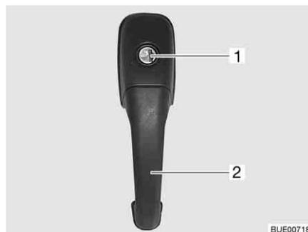
Fig. 29 Door lock of conversion door, outside
