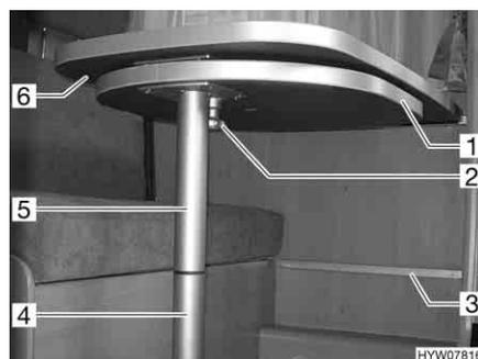
Fig. 76 Suspension table with separable support leg
