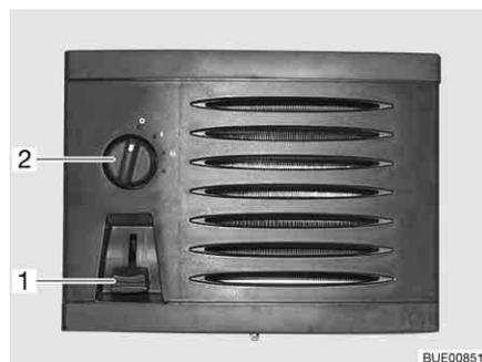
Fig. 185 Operating controls for auxiliary heat exchanger
