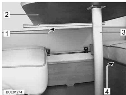
Fig. 82 Suspension table with changeable table leg
