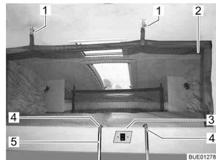
Fig. 95 Pull-down bed complete with applied safety net
