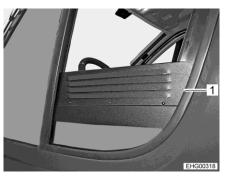
Fig. 78 Forced ventilation grille (side window open)
