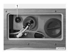
Fig. 123 Water tank with rotary handle
