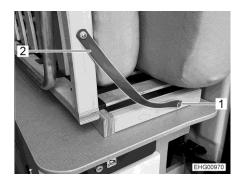
Fig. 70 Retaining strap on the righthand bed base
