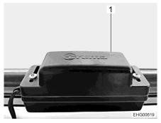
Fig. 112 Window contact switch
