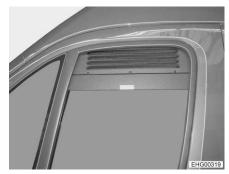
Fig. 79 Forced ventilation grille (side window closed)
