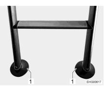
Fig. 84 Plastic plate on the access ladder
