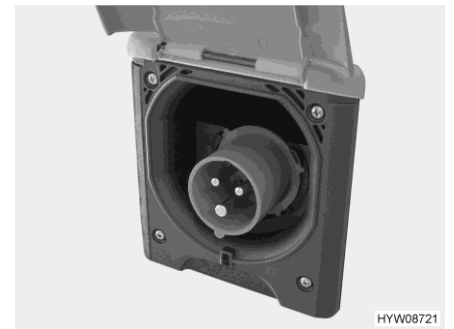
Fig. 73 230 V connection on the vehicle (CEE socket outlet)
