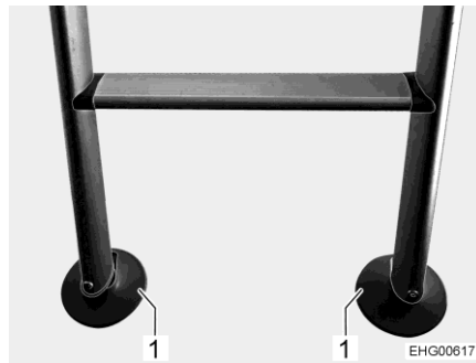
Fig. 59 Plastic plate on the access ladder
