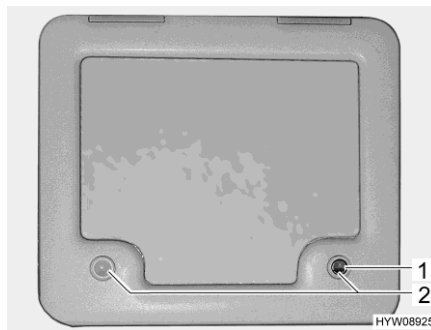
Fig. 107 Flap for the sewage tank
