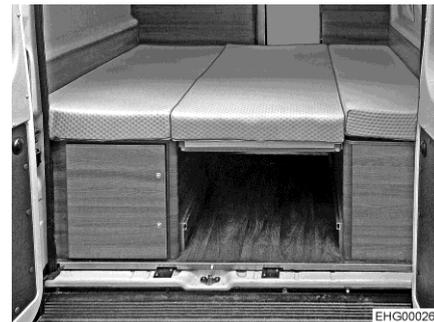
Fig. 41 Transverse rear bed after conversion (variant with 3 longitudinal cushions)
