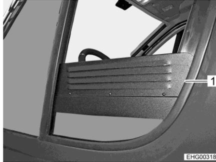
Fig. 53 Forced ventilation grille (side window open)
