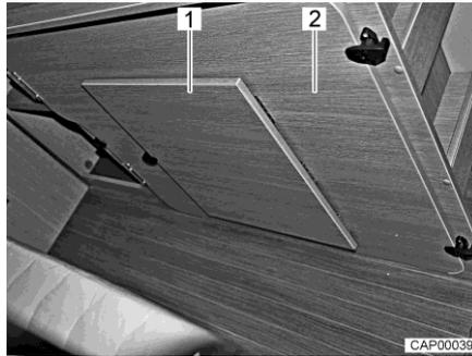
Fig. 50 Removable board on the right-hand bedding box
