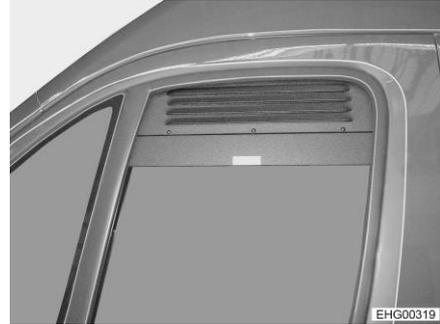
Fig. 54 Forced ventilation grille (side window closed)
