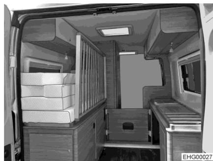
Fig. 48 Transport position (folding bed base)
