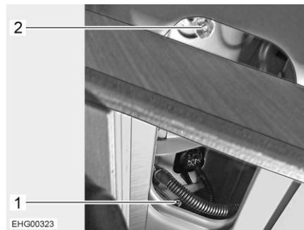
Fig. 110 Fixture of the rear lights unit
