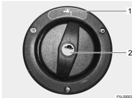
Fig. 93 Cap for the drinking water filler neck
