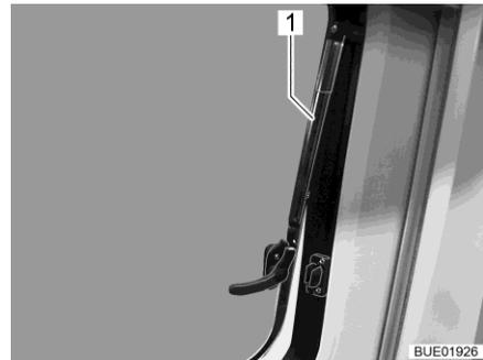
Fig. 12 Hinged window with automatic hinges, open
