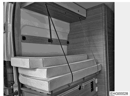
Fig. 49 Transport position (removable bed base)
