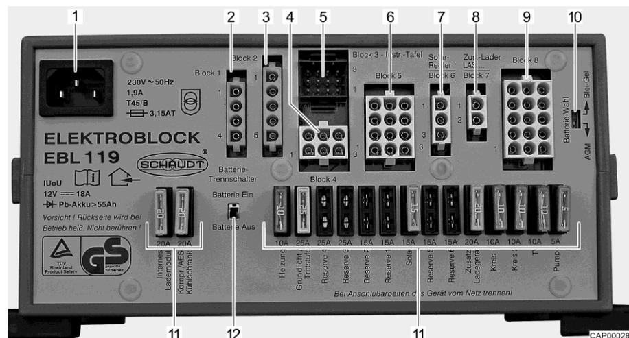
Fig. 69 Transformer/rectifier (EBL 119)
