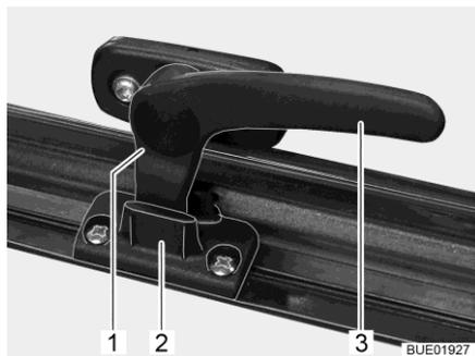
Fig. 13 Catch lever in "continuous ventilation" position
