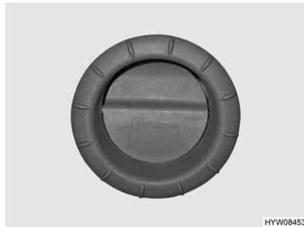
Fig. 53 Air outlet nozzle of the hot-air heater
