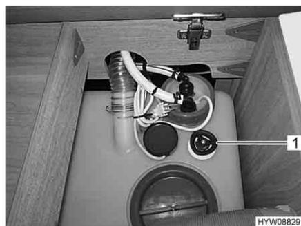
Fig. 72 Water drainage handle
