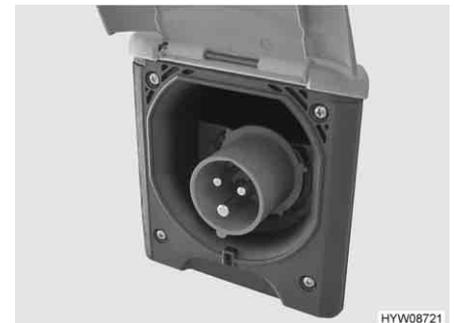
Fig. 44 230 V connection on vehicle
