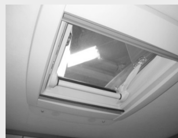
Afb. 42: Dakluik 400x400 mm VisionStar 700x500 mm
