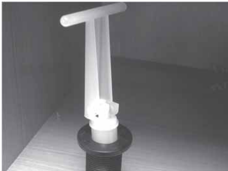
Fig. 88: Drain plug in fresh water tank, open (rocker lever straight)
