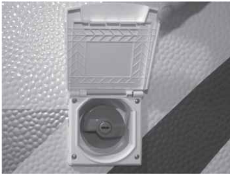
Fig. 76: Fresh water intake port
