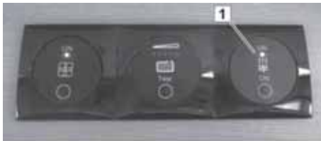
Fig. 75: On-Off switch of the floor heating system
