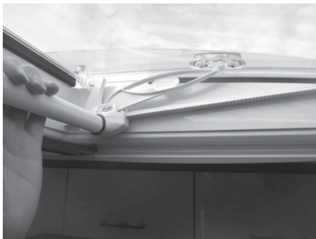
Fig. 102: Operating the MPK skylight
