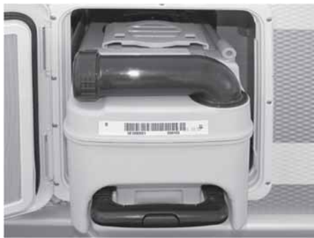
Fig. 40: Waste holding tank
