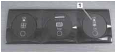
Fig. 111: On-Off switch of the floor heating system
