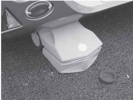
Fig. 90: Wheeled waste water tank
