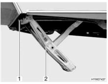
Fig. 23 Corner steady cranked down
