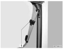
Fig. 58 Hinged window with rotary hinge
