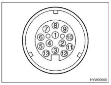
Fig. 131 Contact diagram of the thirteen-pin plug
