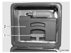
Fig. 196 Sewage tank (example)
