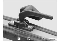
Fig. 61 Catch lever in "continuous ventilation" position
