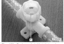
Fig. 192 Drain cock (with rocking lever)
