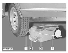
Fig. 194 Waste water tank, mobile
