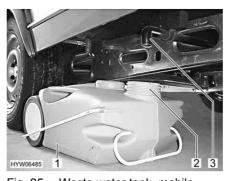
Fig. 25 Waste water tank, mobile
