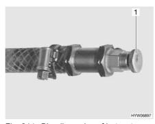
Fig. 214 Bleeding valve of hot-water heater
