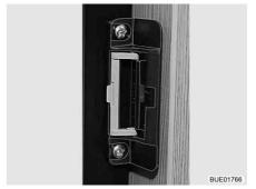
Fig. 187 Locking device in ventilation position
