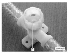
Fig. 160 Drain cock for hot water source
