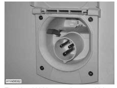
Fig. 125 230 V connection on vehicle
