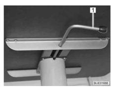
Fig. 76 Lift-off table release
