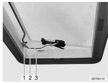
Fig. 69 Heki skylight in ventilation position 2
