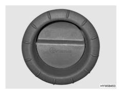
Fig. 138 Air outlet nozzle of the hot air distribution
