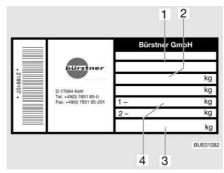
Fig. 227 Vehicle identification plate
