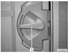
Fig. 30 Door lock of conversion door, inside
