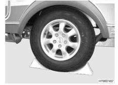
Fig. 230 Securing support wheel
