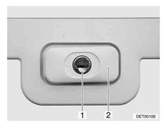
Fig. 35 Flap lock, rectangular, closed
