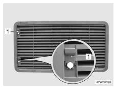
Fig. 173 Refrigerator ventilation grill (with sliding trap)
