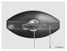
Fig. 33 Flap lock, elliptical-shaped, closed
