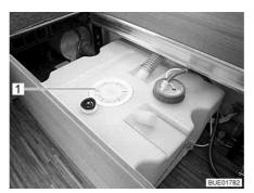
Fig. 207 Cleaning opening of the water tank (example)
