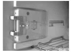
Fig. 183 Locking device in ventilation position
