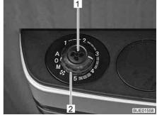
Fig. 144 Knob and rotary switch for fan control
