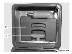
Fig. 205 Flap for the sewage tank
