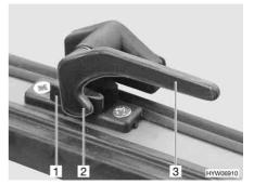
Fig. 57 Catch lever in "closed" position
