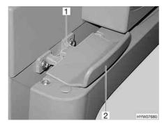
Fig. 184 Lock of refrigerator door, closed (Thetford)
