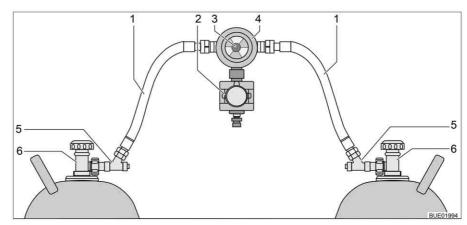
Fig. 113 Gas bottle switching facility with CPU
