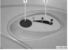
Fig. 204 Flush button/indicator lamp Thetford toilet
