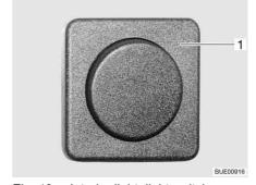
Fig. 48 Interior light, light switch separate from the lamp
