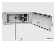
Fig. 111 External gas connection, gas isolator tap closed
