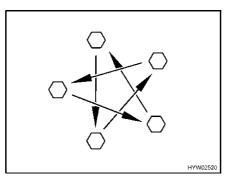
Fig. 228 Tighten the wheel nuts or wheel bolts cross-wise
