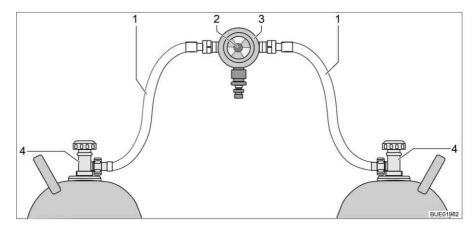
Fig. 112 Gas bottle switching facility
