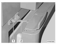
Fig. 185 Refrigerator door in ventilation position (Thetford)
