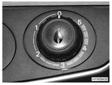
Fig. 143 Hot-air heater control knob
