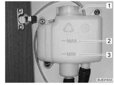
Fig. 213 Compensator reservoir without panel
