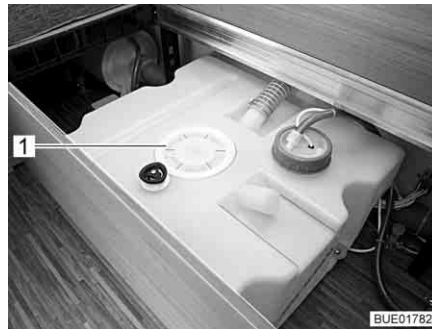
Fig. 205 Cleaning opening water tank
