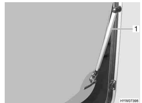
Fig. 56 Hinged window with automatic hinge
