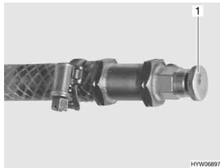
Fig. 214 Bleeding valve of hot-water heater
