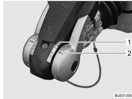
Fig. 7 Check "AKS closed"
