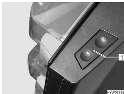
Fig. 180 Release button of the refrigerator door (Dometic 8 series)
