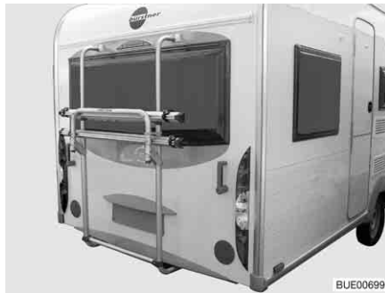
Fig. 13 Bike rack on the rear wall
