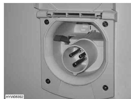
Fig. 121 230 V connection on vehicle
