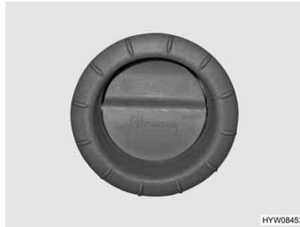
Fig. 134 Air outlet nozzle of the hot air distribution
