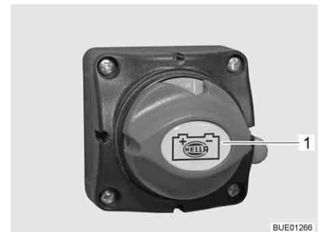
Fig. 115 Battery main switch, "ON" position
