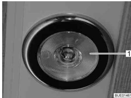
Fig. 48 Recessed light, light switch in the lamp
