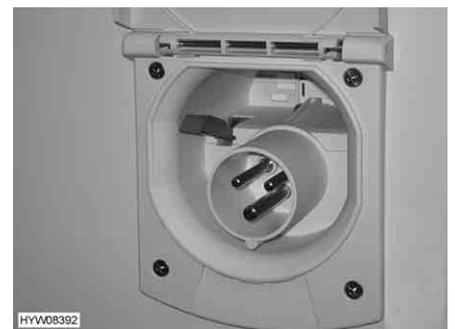
Fig. 121 230 V connection on vehicle
