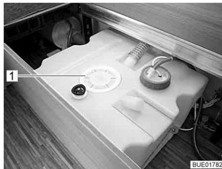
Fig. 194 Cleaning opening water tank
