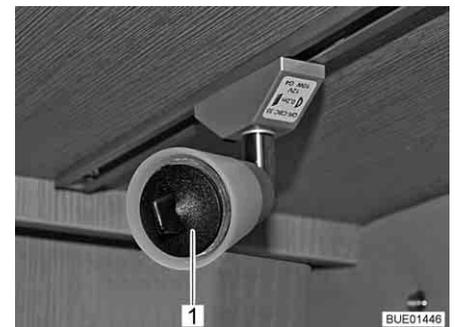
Fig. 212 Suction cup for replacing the lamp
