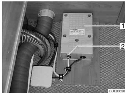
Fig. 143 Transformer for electrical floor warming unit
