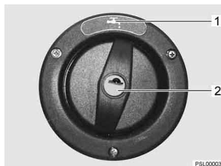
Fig. 39 Cap for the drinking water filler neck
