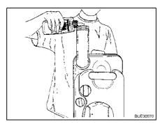
Fig. 190 Filling with sanitary liquid
