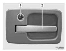
Fig. 25 Door lock of conversion door, outside
