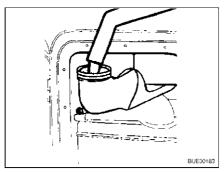
Fig. 204 Filling with fresh water
