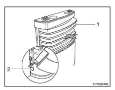
Fig. 144 Heater cover, lower brackets
