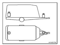
Fig. 8 Incorrect weight distribution
