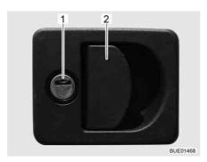
Fig. 30 Flap lock with recessed handle
