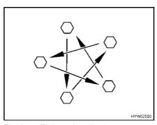
Fig. 245 Tighten the wheel nuts or wheel bolts cross-wise
