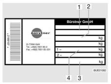
Fig. 244 Vehicle identification plate
