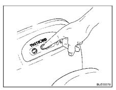
Fig. 197 Opening the sliding trap
