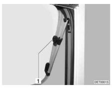
Fig. 55 Hinged window with rotary hinges
