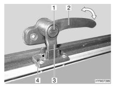
Fig. 61 Catch lever with safety knob in "continuous ventilation" position
