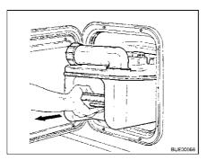
Fig. 215 Removing the Thetford cassette
