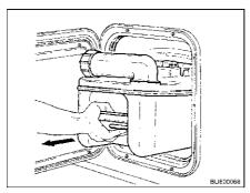
Fig. 199 Removing the Thetford cassette
