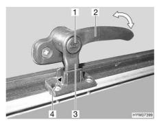
Catch lever with safety knob in Fig. 56 "continuous ventilation" posi-
