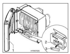
Fig. 136 Removing heater cover
