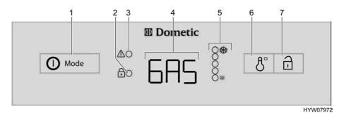
Fig. 171 Operating controls for the refrigerator (Dometic 8 series with AES)
