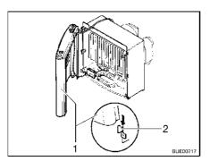
Fig. 138 Heater cover, retaining clips
