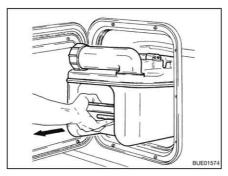
Fig. 188 Removing the Thetford cassette
