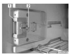
Fig. 175 Locking device in normal position
