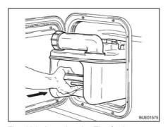
Fig. 191 Inserting the Thetford cassette
