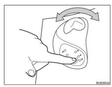
Fig. 214 Operating the flush
