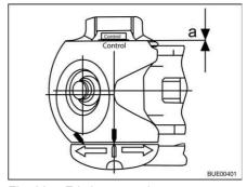
Fig. 223 Friction control
