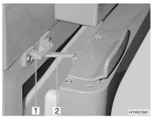
Fig. 178 Refrigerator door in ventilation position (Thetford)
