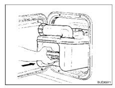
Fig. 202 Inserting the Thetford cassette
