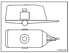
Fig. 9 Correct weight distribution
