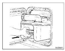
Fig. 218 Inserting the Thetford cassette
