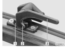
Fig. 53 Catch lever with safety knob in "closed" position
