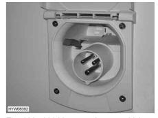
Fig. 122 230 V connection on vehicle
