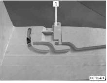
Fig. 69 Ventilation position locking mechanism
