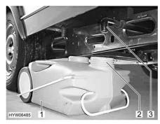
Fig. 22 Waste water tank, mobile
