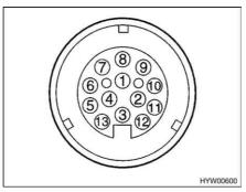
Fig. 127 Contact diagram of the thirteen-pin plug
