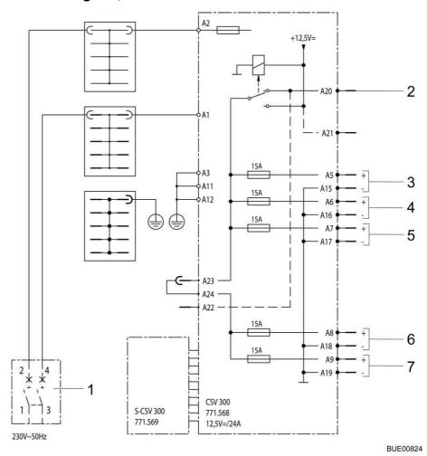
Fig. 131 Circuit diagram, interior (CSV 300)
