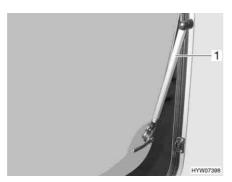
Fig. 60 Hinged window with automatic hinges
