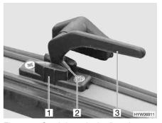
Catch lever in the "continuous Fig. 57 ventilation" position
