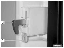
Fig. 174 Lock hook fixture
