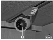
Fig. 241 Suction cup for replacing the lamp
