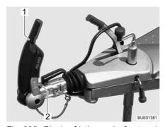
Fig. 225 Display friction pads, front and back
