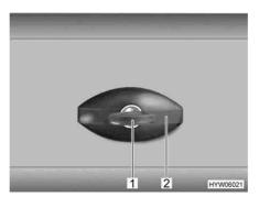
Fig. 29 Flap lock, elliptical-shaped, closed
