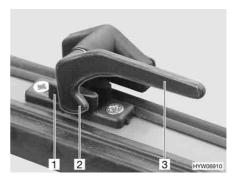
Fig. 58 Catch lever with safety knob in "closed" position
