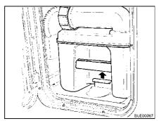
Fig. 206 Pulling the retaining clip
