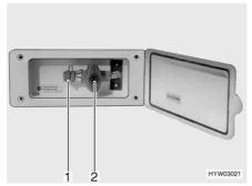
Fig. 113 External gas connection, gas isolator tap closed
