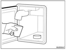
Fig. 220 Emptying the fresh water filler neck
