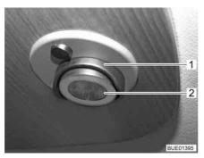
Fig. 232 Recessed halogen light
