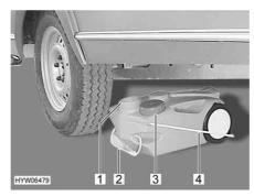
Fig. 184 Waste water tank, mobile
