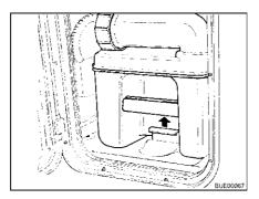
Fig. 187 Pulling the retaining clip
