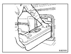
Fig. 207 Removing the Thetford cassette
