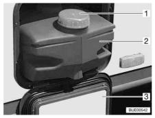
Fig. 180 Water tank 22 I
