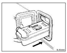
Fig. 210 Inserting the Thetford cassette
