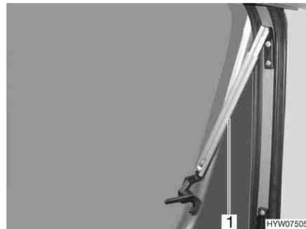
Fig. 53 Hinged window with automatic hinges, open
