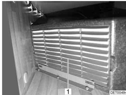
Fig. 206 Air conditioning unit (Truma)
