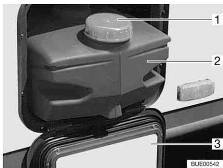
Fig. 163 Water tank 22 l
