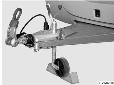
Fig. 230 Securing support wheel
