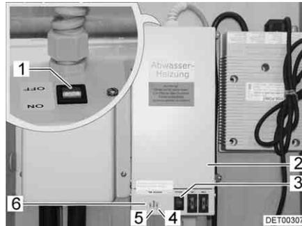
Fig. 131 Transformer with control unit
