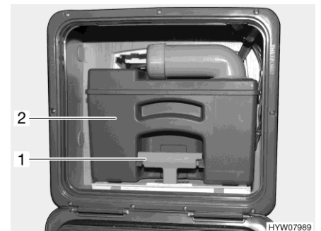
Fig. 269 Sewage tank (example)
