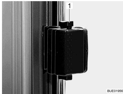
Fig. 102 Sliding window, locked
