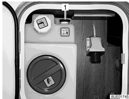
Fig. 254 Water tank (service unit)
