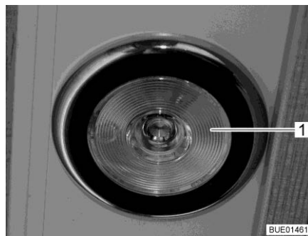
Fig. 79 Recessed light, light switch in the lamp
