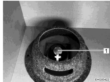
Fig. 85 Active docking station on shelf above the driver's cabin
