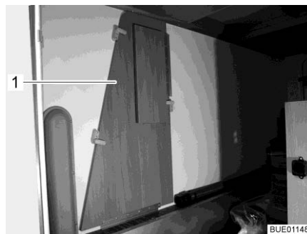
Fig. 13 Bed widening in the rear garage
