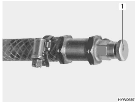
Fig. 287 Bleeding valve of hot-water heater
