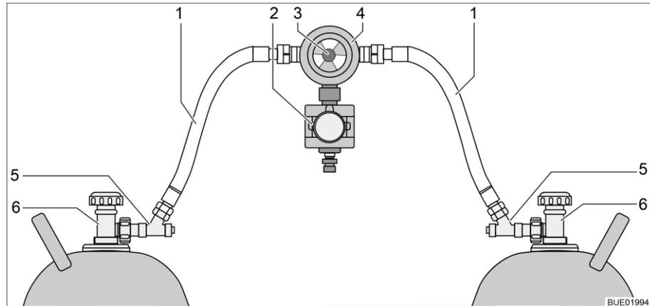
Fig. 12 Gas regulator with CPU and hose break guard
