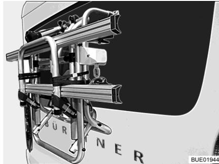
Fig. 3 Bike rack, folded upwards
