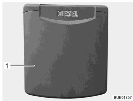
Fig. 40 Fuel filler neck external flap
