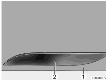
Fig. 60 Pressure lock, closed
