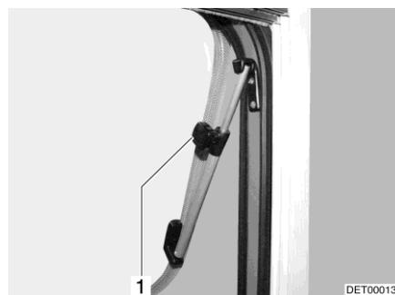
Fig. 79 Hinged window with rotary hinge
