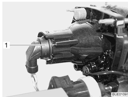
Fig. 163 Low beam/main beam/parking light
