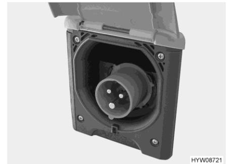
Fig. 114 230 V connection on the vehicle (CEE socket outlet)
