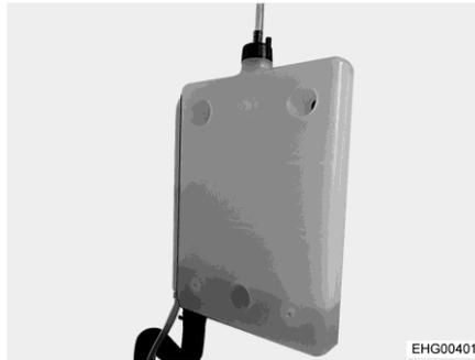
Fig. 159 Compensator reservoir
