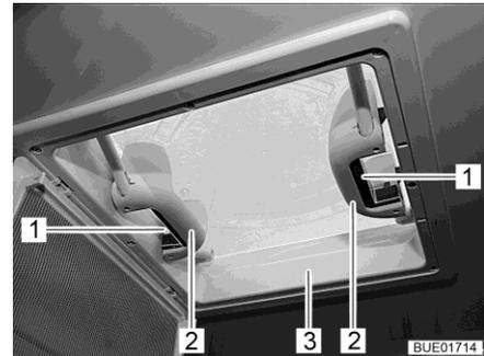
Fig. 91 Handles with snap latches
