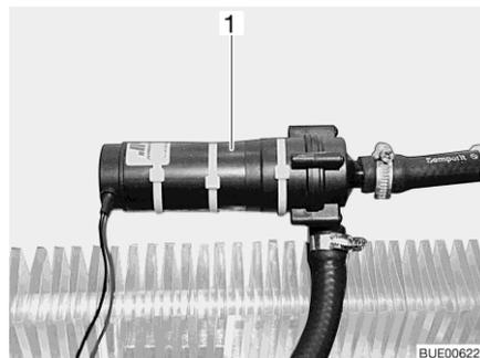
Fig. 134 Auxiliary circulating pump
