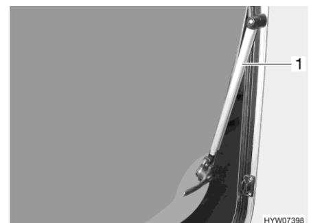
Fig. 80 Hinged window with automatic hinge
