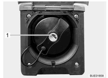
Fig. 41 Cap for the fuel filler neck
