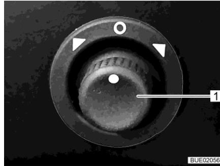
Fig. 29 External mirror adjustment switch
