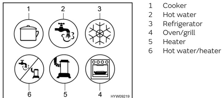
Fig. 127 Possible symbols for the gas isolator taps
